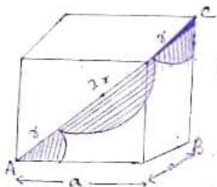
Geometry of a BCC unit cell
